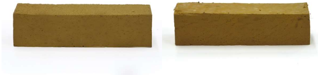
Figure 3 Base coat (left) and Top coat (right) clay plaster specimens
