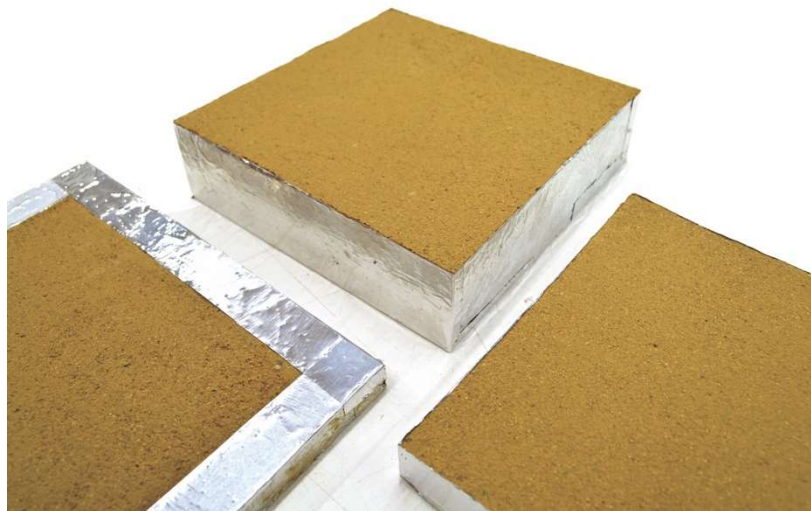
Figure 4. Clay moisture buffering specimens of different thicknesses
