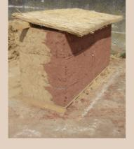
The current confident use of cob in new building is of great interest in reducing energy expend and CO2 emissions during construction. But this performance does not meet current in-use the regulations. CobBauge, through the study of different plant fibers, the characteristics of different soils, seeks to give the keys to an optimization of the mixes and implementation processes ma cob compatible with the regulations, economically more affordable, technically and aesthetical more acceptable.
